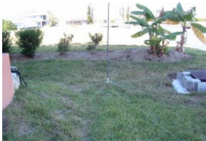
Assembled antenna focusing on the base and radials
