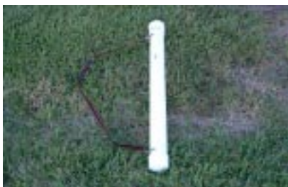
The carrying case made from 4" PVC pipe. The antenna is fairly fragile and this protects it nicely.
