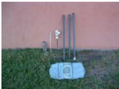
The carrying case made from 4" PVC pipe. The antenna is fairly fragile and this protects it nicely.
